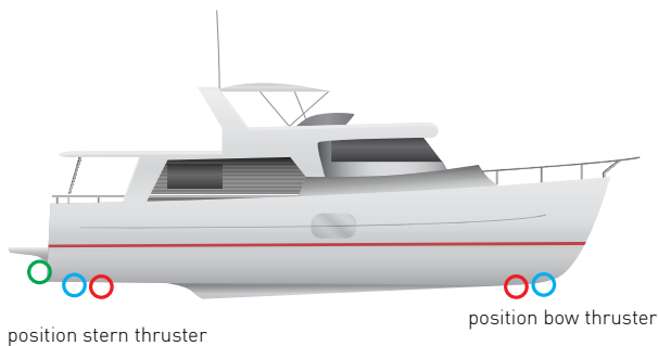
Fig. 7: mounting displacement hull boat
