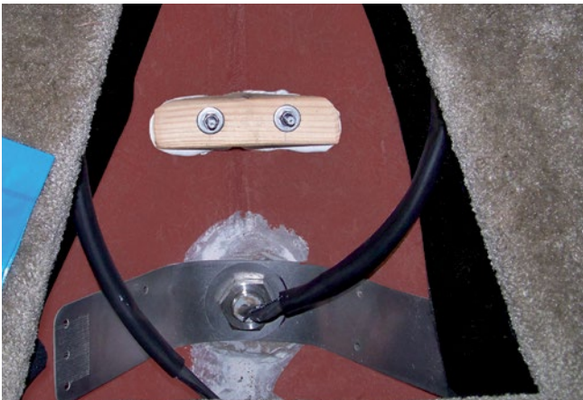
Fig. 25: Screw connection GRP in the boat interior
