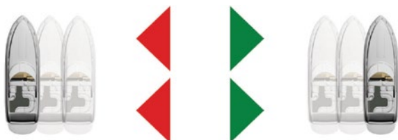
Fig. 39: bow and stern thrusters combined
